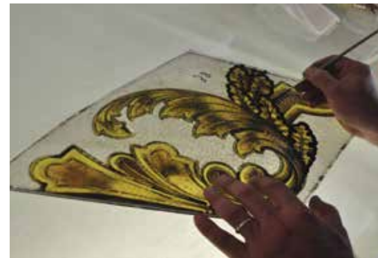
2. The glass blank is placed on top of the original and the dark lines are traced with a brush by hand.
